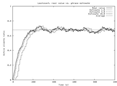
**Figure 4:** Dynamic tracking of over a random tree of height 8 with 279 potential receivers.
