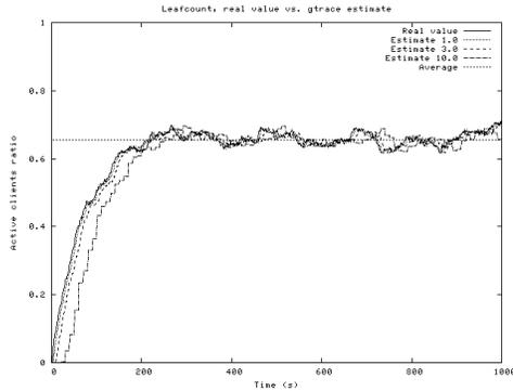
**Figure 5:** Dynamic tracking of gTrace over a full binary tree of height 9 with 512 potential receivers.
