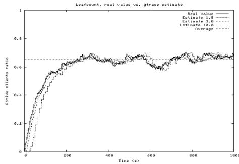
**Figure 1:** Dynamic tracking of gTrace using update period of 1, 3 and 10 seconds, over a full binary tree of height 8.
