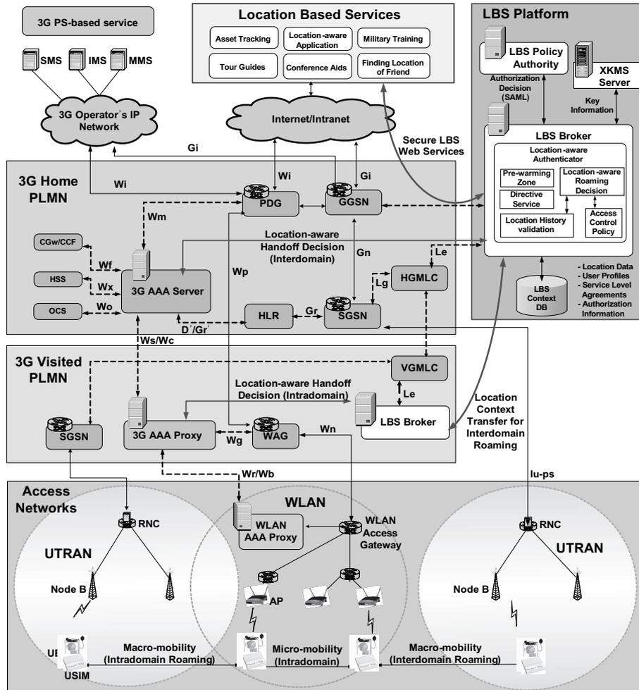
Wr/Wb: This interface carries AAA signaling between the WLAN and the 3G visited or home PLMN in a secure manner
