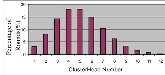
**Fig. 1.** CH Number Distribution of LEACH (100 nodes, Target CH Number =5. The percentage of CH number greater than 12 is negligible)
