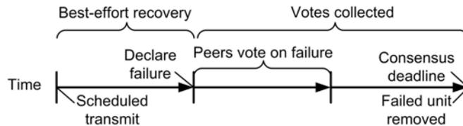
**Fig. 4.** Timeline for best-effort *ACK* recovery, peer voting, and peer consensus to remove a node that failed to transmit its scheduled *ACK*
