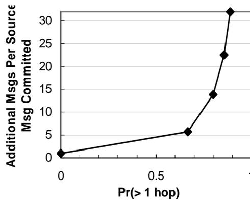
**Fig. 8.** The additional packet overhead required, as a function of the probability that any given group member is greater than one hop from the original message or *ACK* source
