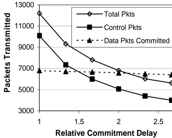
**Fig. 7.** Total number of data and control packets transmitted during a simulation run, as a function of the relative commitment delay
