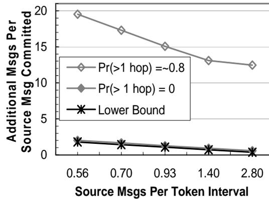
**Fig. 6.** Protocol efficiency as a function of traffic rate
