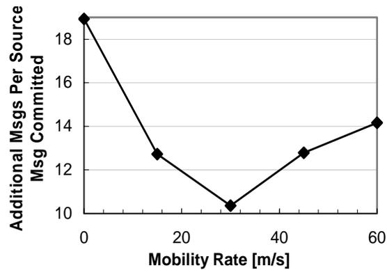
**Fig. 9.** Protocol packet overhead as a function of node mobility rate using a random waypoint model and zero pause time
