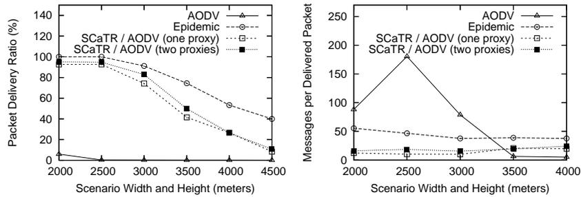
**Fig. 1.** Delivery ratio (left) and signaling overhead (right) for the scheduled routes mobility model with varied network connectivity.
