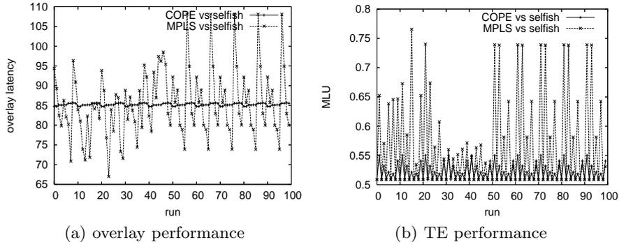
**Fig. 3.** MPLS and COPE with selfish overlay. 14-node topology with a 4-node overlay network, overlay fraction = 10%, load scale factor = 0.5. (MLU: Maximum Link Utilization)
