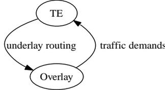
**Fig. 1.** vertical interaction game: TE determines the physical routing, which decides link latency experienced by overlay. Given the observed latency, overlay optimizes its logical routing and changes the physical traffic demands, which, in turn, affects the underlay routing.
