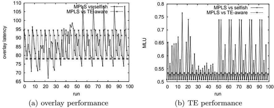
**Fig. 4.** TE-aware overlay and selfish overlay on MPLS. 14-node topology with a 4-node overlay network, overlay fraction = 10%, load scale factor = 0.5 (MLU: Maximum Link Utilization).
