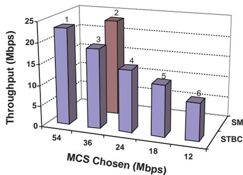
**Fig. 6.** MIMO LA selected at different locations and the throughput achieved in an outdoor environment
