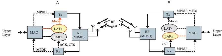
Fig. 4. Structure of MIMO LA Algorithm
