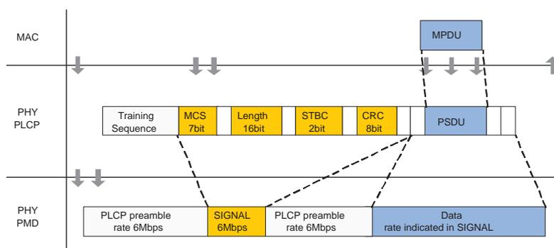
**Fig. 3.** Packet Receiving Procedure
