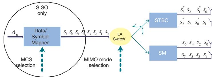
**Fig. 1.** Challenge of Link Adaptation in 802.11n ( $2 \times 2$ )
