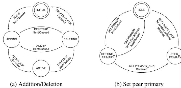
Fig. 3. State transition diagram for local addresses.
