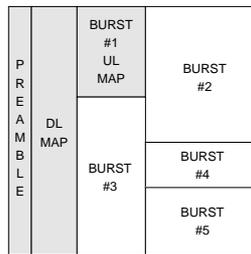
**Fig. 2.** OFDMA Downlink subframe structure in IEEE 802.16.
