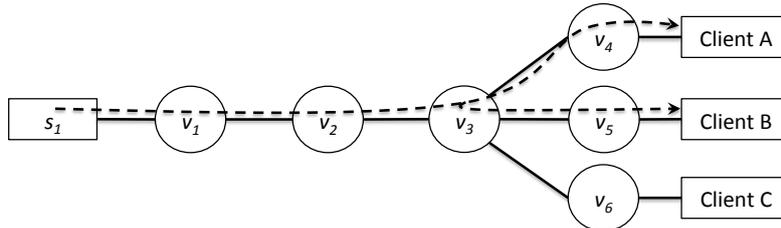
**Fig. 2.** An example topology with optimal caching location at  $v_3$ .
