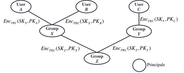
Fig. 6. Principal hierarchy and encryption of principals' private keys, where  $Enc_{PKC}$  is the function of encryption via a certain public key cryptographic algorithm,  $PK_i$  is the public key of principal  $i$ , and  $SK_i$  is the private key of  $i$ .
