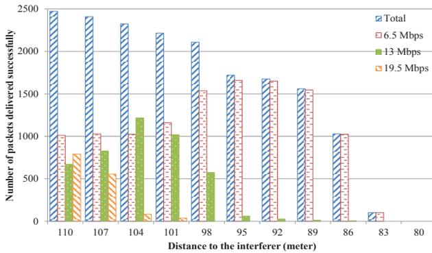
Fig. 6: The number of packets successfully delivered by  $L_{AP_1,MS_2}$  at three different data rates (6.5, 13 and 19.5 Mbps) under the interference from  $L_{AP_3,MS_4}$  and with a 6 Mbps traffic load.
