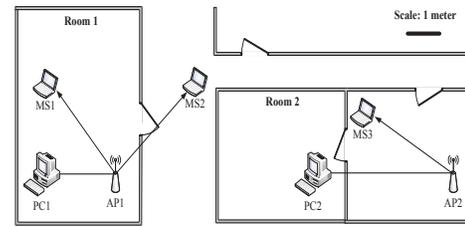
**Fig. 1: The topology of the testbed consists of two APs and three mobile stations.**
