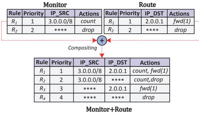
Fig. 2. Example of parallel composition, adapted from [16]
