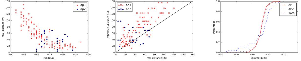
(a) RSS vs Actual Distance to APs from Observation Points (b) Actual Distance vs Estimated Distance to APs (c) Percentage of Spheres that include APs
