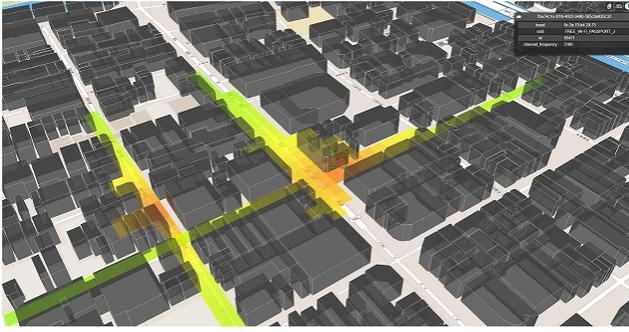
Fig. 1. Wi-Fi Radio Map Visualization (around Yodoyabashi, Osaka City)
