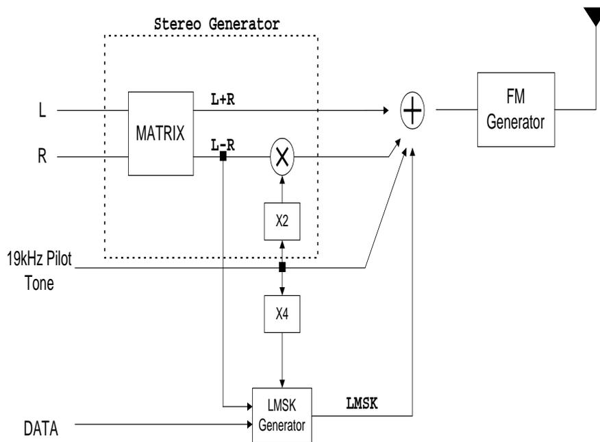
Fig. 1 The block diagram of the DARC system
