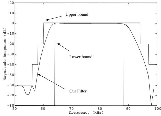
Fig. 2 Filter requirement of the DARC system and the Chebyshev type-2 filter
