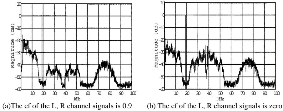
Fig. 3 Base-band frequency spectrums of the ordinary FM signals and DARC signal
