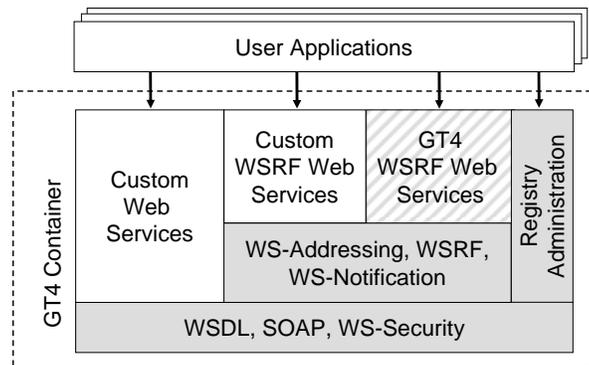
**Figure 5: Capabilities of a GT4 container**
