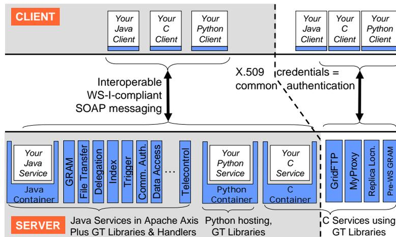
**Figure 1: GT4 architecture schematic, showing many (but not all) components. Shared boxes denote GT4 code; white boxes represent user code**
