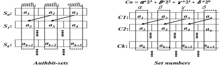
Fig.1. *Authbit sets* and *Set numbers* generation mechanism
