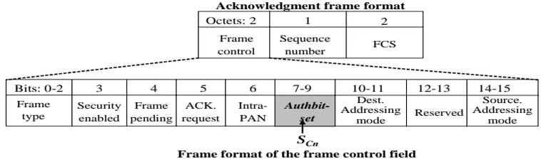
Fig.4. Frame format in the IEEE 802.15.4 Standard
