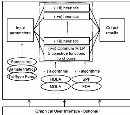
Figure 2. MatPlanWDM toolbox structure.
