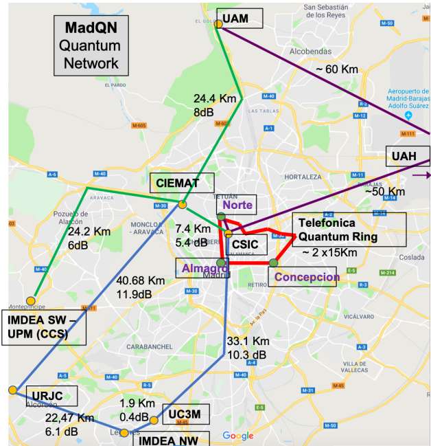
Fig. 2. The Madrid Quantum Network has currently 13 links. The network is a real world one in the sense that all the network is in production facilities and that most of the nodes are being used simultaneously for classical communications, including the fiber. This is not an ad hoc network built for quantum purposes. As a result, this presents the same challenges that a commercial deployment of QKD technologies would need to overcome, making for a realistic testbed. Distances and losses are also representative of a typical metropolitan area network, ranging from 2 to about 40 km and from 3 to 14 dB, respectively (when all losses, not only the fibre is taken into account). Distances and losses (only fiber) are quoted in the figure. The purple lines (connecting to UAH) are under commissioning. The red ring in the center is the old Madrid Quantum Network installed in Telefónica premises [20]. It is interesting to note that some nodes host special installations that are of particular interest, like IMDEA Networks (IMDEA-NW) which hosts a Telefónica 5G lab.
