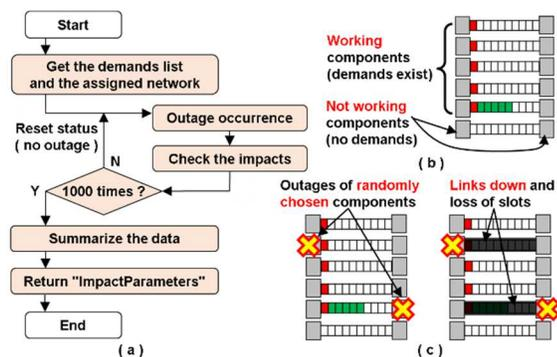
Fig. 4. (a) Outage simulation diagram, (b) Working/not working components, (c) Outages and link downs
