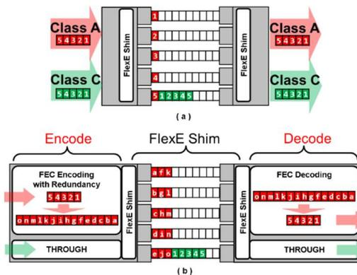
Fig. 1. (a) Conventional FlexEthernet accommodation, (b) Proposed scheme
