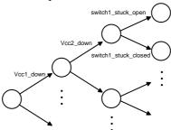
The diagram shows a part of the generated state space. Nodes represent failure states, edges represent component faults and are labelled with the fault identifier. By replacing the edge labels with the associated failure rates, the event graph can be analysed as a Markov-Chain to calculate the state probabilities.
