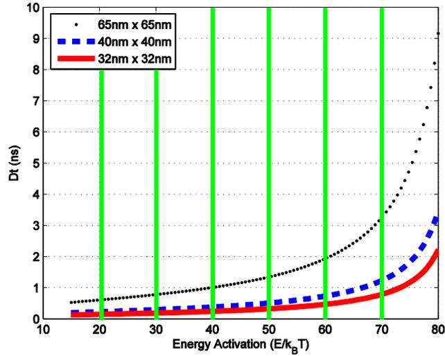
Figure 5: Relationship between switch duration  $Dt$  and  $\xi$ .  $Dt$  can be reduced greatly with low  $\xi$  (e.g. 35) while keeping the same  $I_{switch} = 300\mu A$ . The speed can be further improved by scaling down MTJ size.
