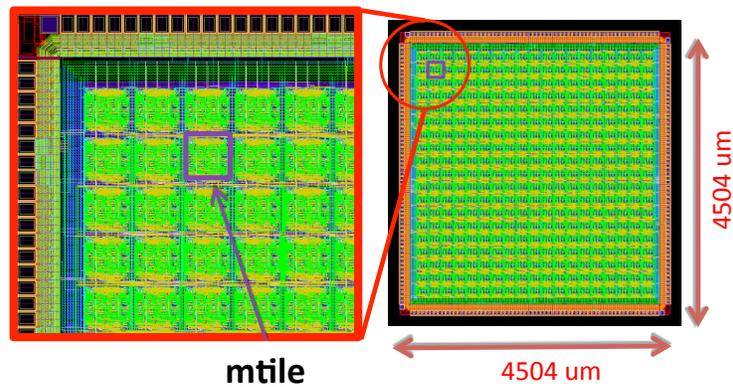
Figure 11: Magnetic FPGA Core Layout
