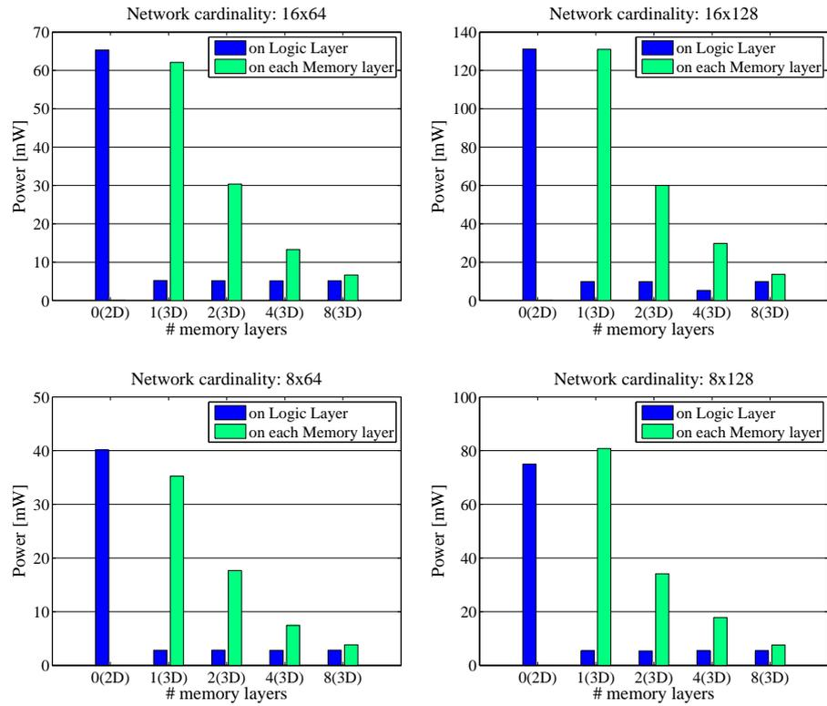
**Fig. 9.** Dynamic power consumed by the Stall/Valid Network on the logic layer (blue) and dynamic power consumed by the data Network on each memory layer (green) for different number memory layers stacked on top of the logic layer.
