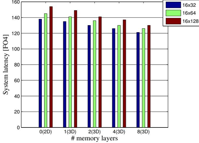
Fig. 10. System latency: Network delay plus memory access time.
