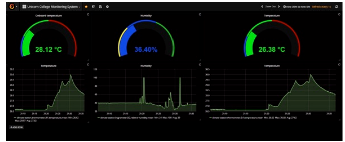
Fig. 7. Main Dashboard with graphical charts and data history for each of the three sensors
