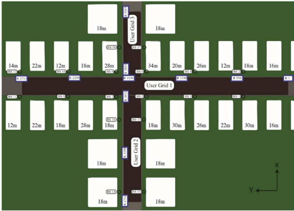
Fig. 1. A 2D example of the system, representing the real life MIMO environment with two main streets, buildings, 18 Base stations and the users along the streets. [10]
