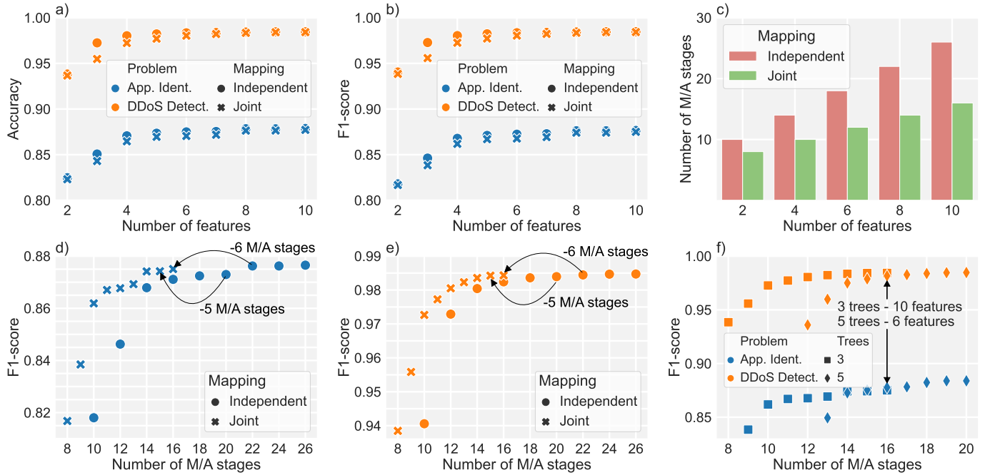
Fig. 4. a) Accuracy, b) F1-score and c) number of M/A stages vs. number of features for independent and joint feature-mapping and for Application Identification and DDoS Detection (3 trees per model); d-e) F1-score for Application Identification (d), and DDoS Detection (e) vs. number of M/A stages for independent and joint feature-mapping (3 trees per model); f) F1-score vs. the number of M/A stages with 3 and 5 trees per model and joint feature-mapping.
