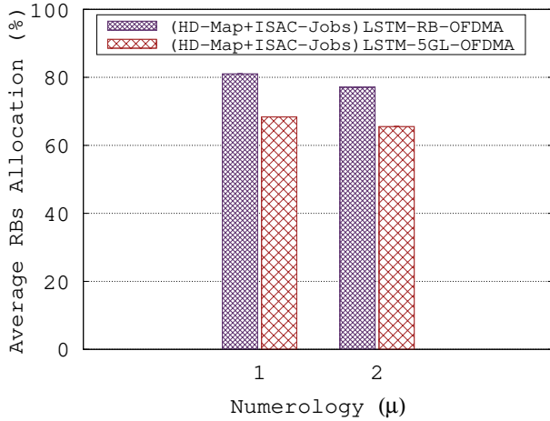
Figure 5: RBs allocation ratio with respect to SR-based-RR scheme by varying numerology for V = 15 with V_{speed} = 60 kmph where L = 60 bytes and CG_w = 15 .
