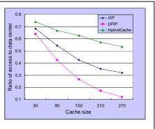
Figure 2: Ratio of access to data center vs. cache size
