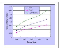
Figure 4: Request failure ratio vs. pause time
