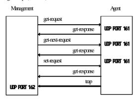
Figure 1. Five types of SNMP Operation
