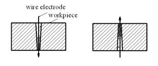
(a) Moving from top to down (b) Moving from down to up **Fig.5.** Wire-cutting back and forth.
