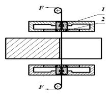
Fig.4. The positioning of guiders with wear properties. (1-Guiders; 2-Spray nozzle plate)
