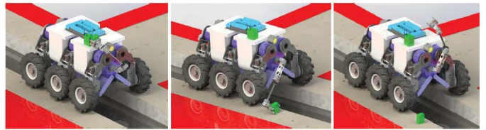
Fig. 3. SIAR Robot deploying one wifi communication repeater.
