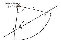
**Fig. 1.** Number of frames F produced by a single sensor node upon detection is  $F = K \frac{D_{AB}}{V}$  where K, V and  $D_{AB}$  stands for the camera frame rate, target speed and pathlength respectively. The pathlength  $D_{AB}$ , in turn, depends on the sensing radius R and the FoV,  $\alpha$ .
