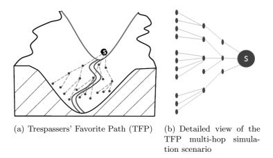
Fig. 3. Deployment Scenario. Intruders follow the favorite path in which the sensors are deployed more densely.
