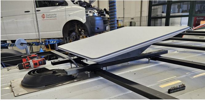
Fig. 5: The Starlink dish mounted on the roof rack.
