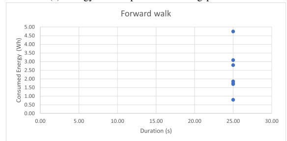
(d) Energy consumption in the forward walk at a constant speed of 0.4 m/s.
