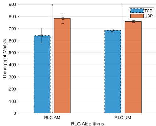
Fig. 3. Average throughput and confidence interval for different RLC configurations for good RSRP condition ( $-76$  dBm).
