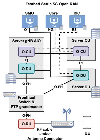
Fig. 1. Topology of 5G Open RAN testbed.
