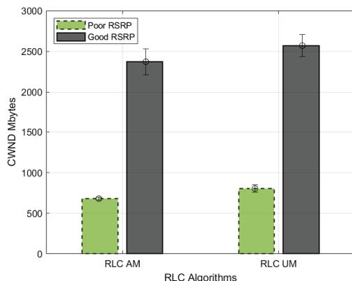
Fig. 5. Average CWND and confidence interval using TCP protocol for different RLC configurations and RSRP conditions.
