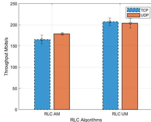
Fig. 4. Average throughput and confidence interval for different RLC configurations poor RSRP condition ( $-115$  dBm).
