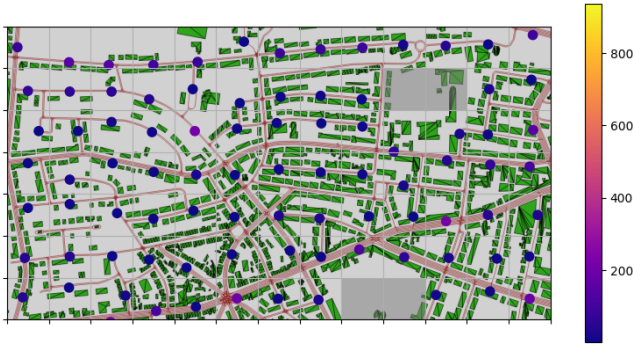
Fig. 3: Uniform placement. The points are distributed uniformly to cover the largest portion of the area, but the samples per point are very low.
